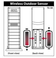
The Outdoor Sensor is weather resistant, but not water proof. To ensure maximum Sensor life, mount it in a covered place out of the elements like under the eaves. Placement on the North side of your home will provide the most accurate readings. Mount it about 18" down from the eaves for optimum performance. This ensures that the weather data collected by the Outdoor Sensor will not be affected by the temperature of the air leaving the attic.
