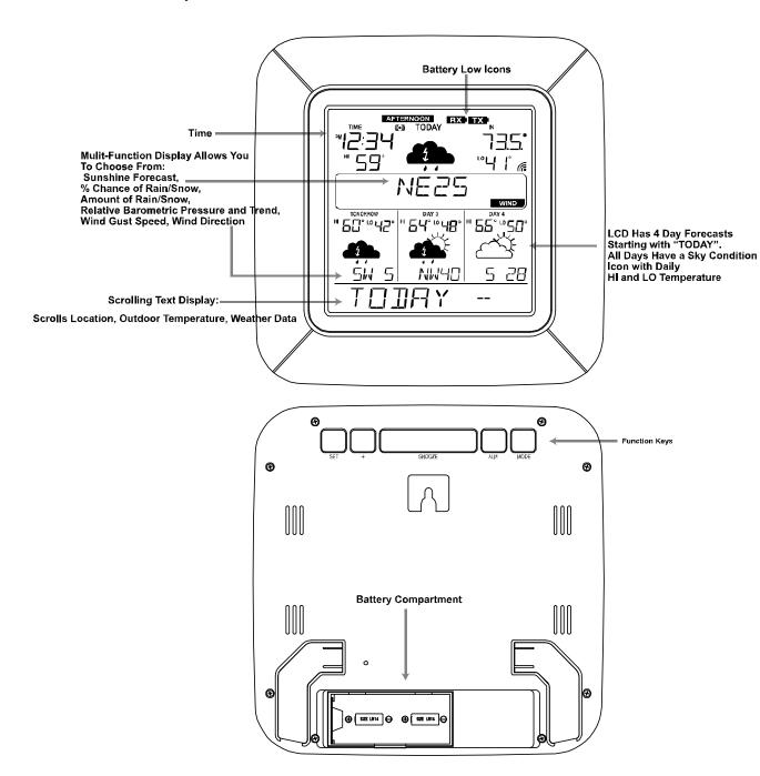
Press the "SNOOZE" Key to cycle through the type of detailed weather information that will display below the forecast icons:
