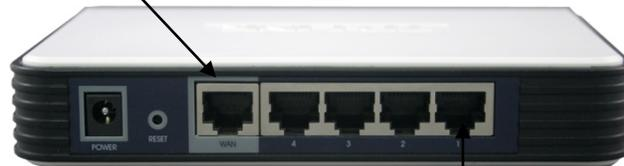
4. Lastly another RJ-45 cat5e network cable plugs into a LAN port on the router at one end, and the other end plugs into your Ethernet →
